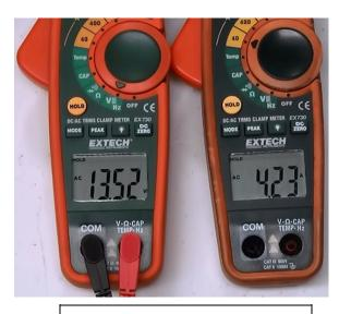
AC output 13.52 x 4.23 = 57.19 watts.
