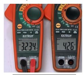
AC input to coil & at load  $32.34 \times .4.26 = 137.8 \text{ watts.}$
