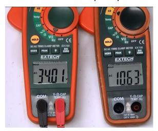
AC input to coil & B4 rectifier  $34.01 \times .10.63 = 361.53$  watts.
